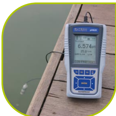
Waterproof Meter and Electrode for Harsh Outdoor Measurements
